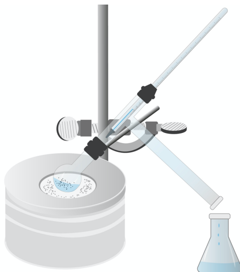
Figure 1 Microscale simple distillation set-up with air condenser
