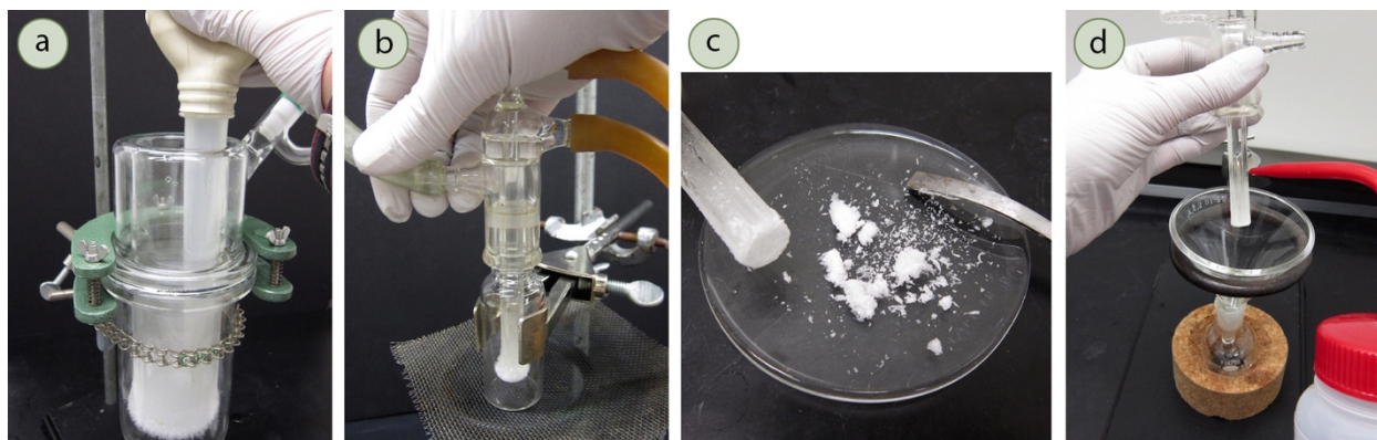
Figure 6.36: a) Removing ice water from the cold finger using a turkey baster, b) Releasing the pressure after the sublimation, c) Scraping the crystals from the cold finger, d) Rinsing the cold finger into a round bottomed flask for later evaporation.
