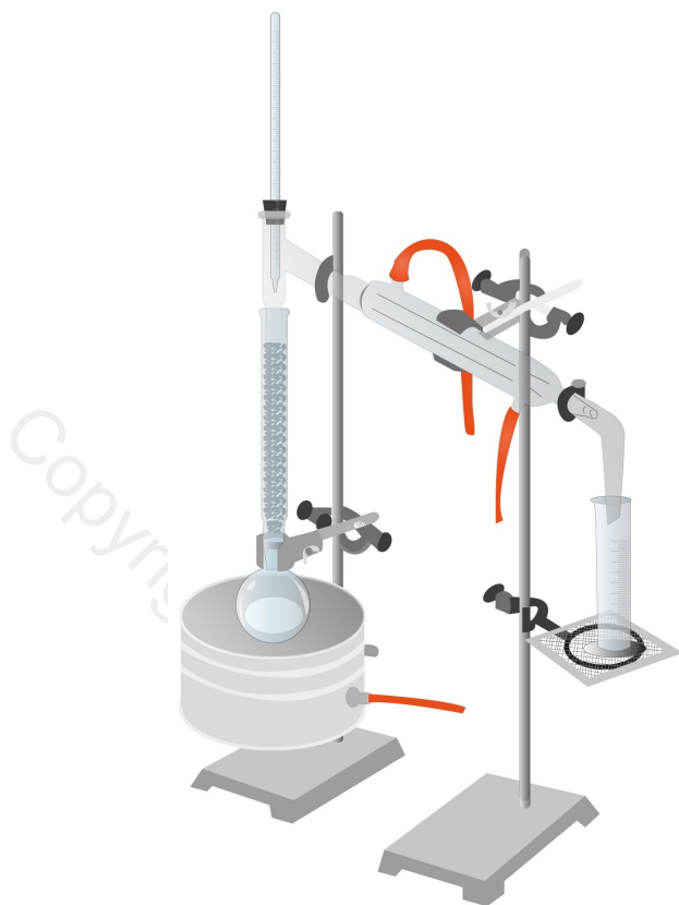
Figure 1 Fractional distillation set-up with fractionating column above the sample flask
