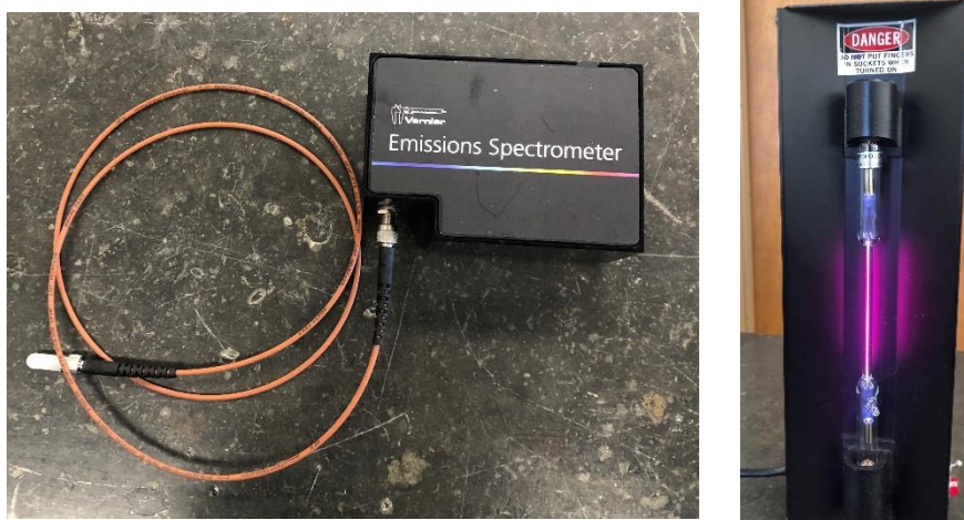
Figure 2.2. Vernier emission spectrometer, optical fiber, and hydrogen tube.
