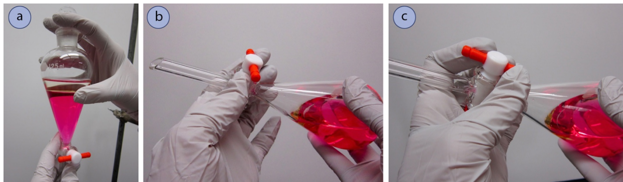
Figure 4.26: a) Holding the separatory funnel before shaking, b) Inverting the funnel to mix the components, c) Venting to release pressure.
