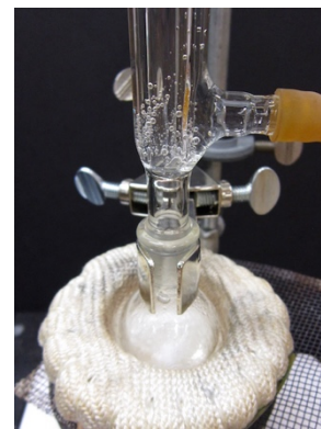
Figure 4.5: Reaction to make isopentyl acetate.
